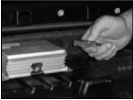
STEP 20 Remove the plug from the factory amplifier.
